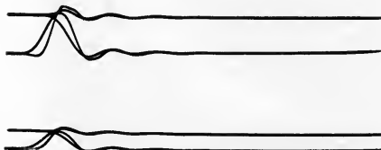
Fig. 13. Normal and crispened step waveforms for a system of 2-mc bandwidth to the 3-db point.
